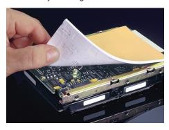
Gap Pad® VO is a cost-effective, thermally conductive interface material. The material is a filled, thermally conductive polymer supplied on a rubber-coated fiberglass carrier allowing for easy material handling. The conformable nature of Gap Pad® VO allows the pad to fill in air gaps between PC boards and heat sinks or a metal chassis.
