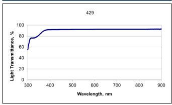
Measured at 0.03 mm [0.001in] per DSTM-501<sup>‡</sup>
