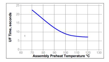
**Note:** Use for estimate only. Data generated on Glass to Glass slide assembly with 180 micron gap, time is to flow a distance of 1 cm.
