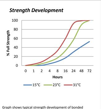
components. An increase of 8°C in temperature will halve the cure time. Lower temperatures will result in a slower cure time.
