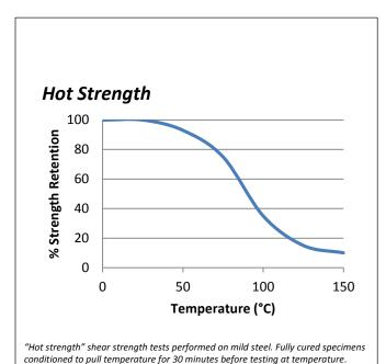
MT3821 can withstand higher temperatures for brief periods (such as for paint baking and wave soldering processes) providing the joint is not unduly stressed. The minimum temperature the cured adhesive can be exposed to is -40°C (-40°F) depending on the materials being bonded.
