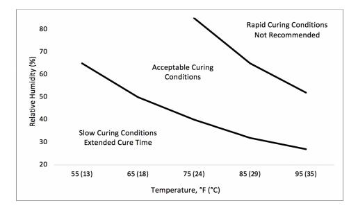
Aeroglaze Z307 coating cures to a tack-free surface in 2-3 hours at 25°C (77°F) and 50% relative humidity. Room temperature cure times of 12 hours permit handling.
