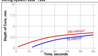
Curing System: Electrodeless, H bulb
