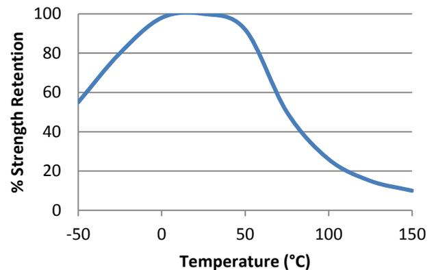
"Hot strength" shear strength tests performed on mild steel. 24hr cure at room temperature and conditioned to pull temperature for 30 minutes before testing.
