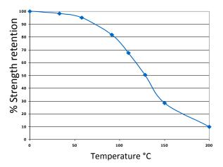
4UV80 can withstand higher temperatures for brief periods (such as for paint baking and wave soldering processes) providing the joint is not unduly stressed. The minimum temperature the cured adhesive can be exposed to is -55°C (-67°F) depending on the materials being bonded.
