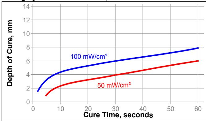
**Curing System: Electrodeless, H bulb**
