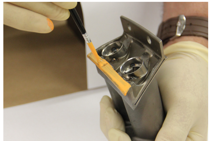
Orange Stop-Off brushed on vane segment
