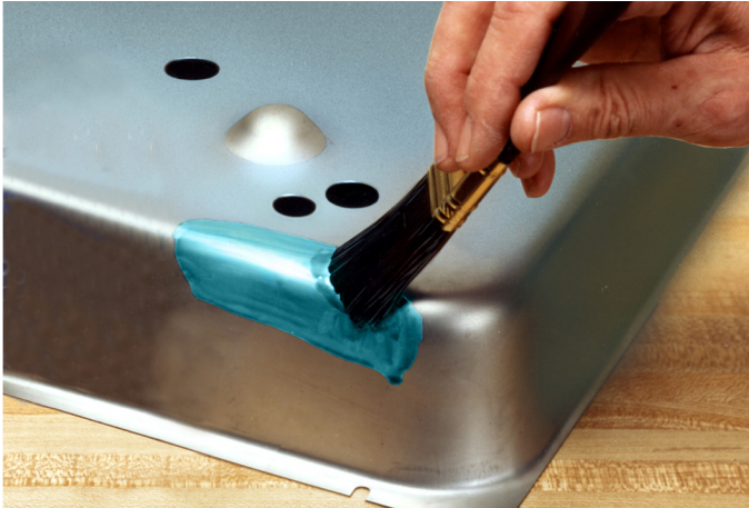
Blue Stop-Off brushed onto surface part
